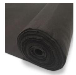
**Abmat**<sup>™</sup> Geo-Fabric is constructed of needle punched Polyester short filaments. These filaments form a stable matrix exhibiting excellent strength and hydraulic characteristics, allowing this product to be used for numerous situations where an economical solution is required for filtration and soil stabilisation in domestic landscaping applications.
